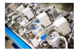
Chemspeed platform equipped with 36 reactors for liquid phase testing at ambiant pressure
